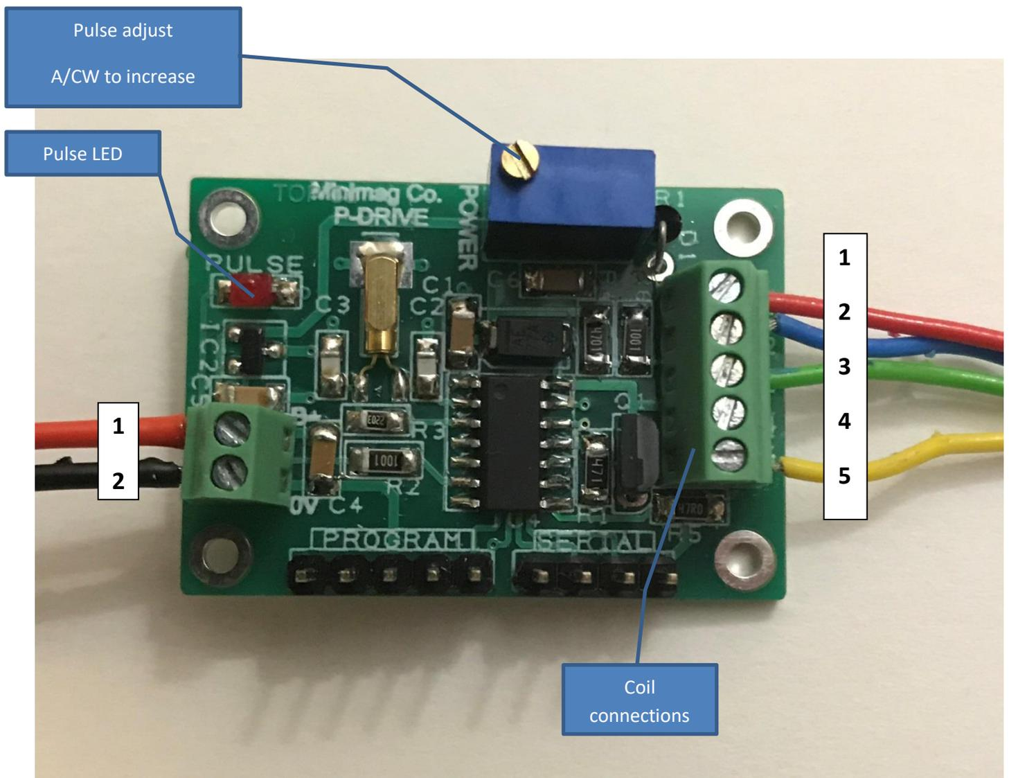
Photo showing connections to the P-Drive circuit board.
