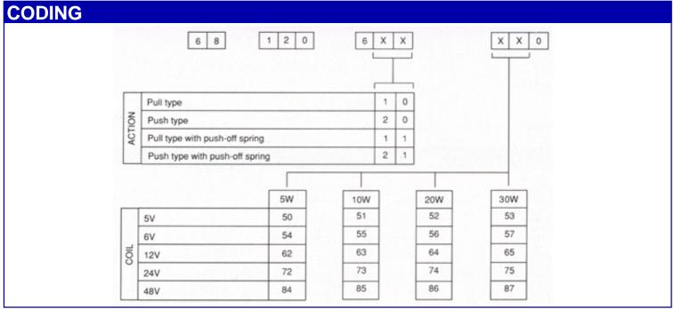
Coil Resistance, Calculate  $R = \frac{V^2}{W}$
